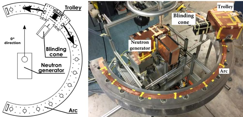
Figure 12. Drawing of arc and trolley setup from above (left) and photo of the setup (right).
