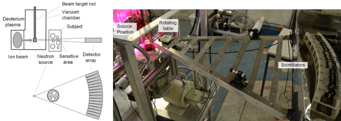
Figure 5. Schematic of imaging setup (left) and a photo of the prototype detector array (right).
