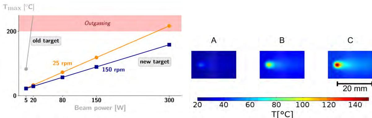
Figure 3. Maximum temperature for different rotation speeds and beam powers (left), and surface temperature distributions (right) for 220 RPM at 70 W (A), 200 W (B), and 300 W (C)
