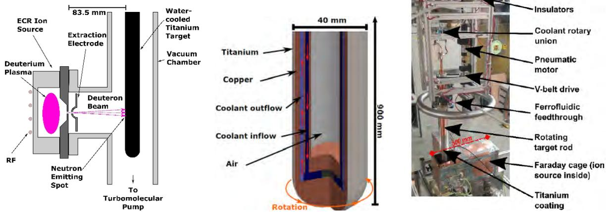
**Figure 2. Schematic of D-D generator operating principles (left), drawing of rotating beam target (middle), and photo of rotating target setup (right).**
