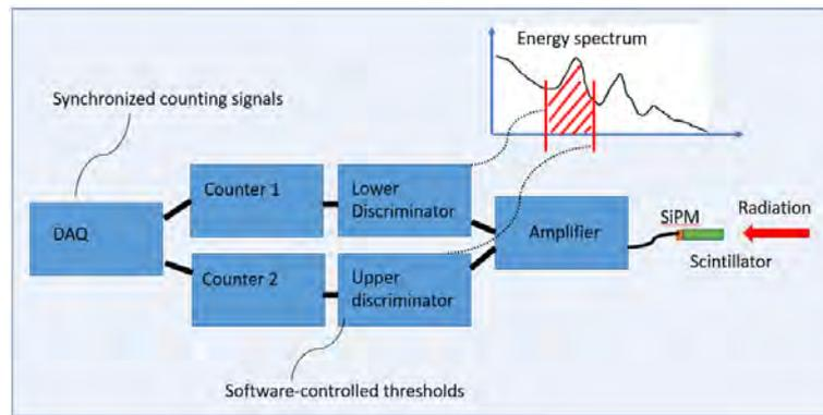
Figure 7. Schematic of pulse processing chain for a single detector.
