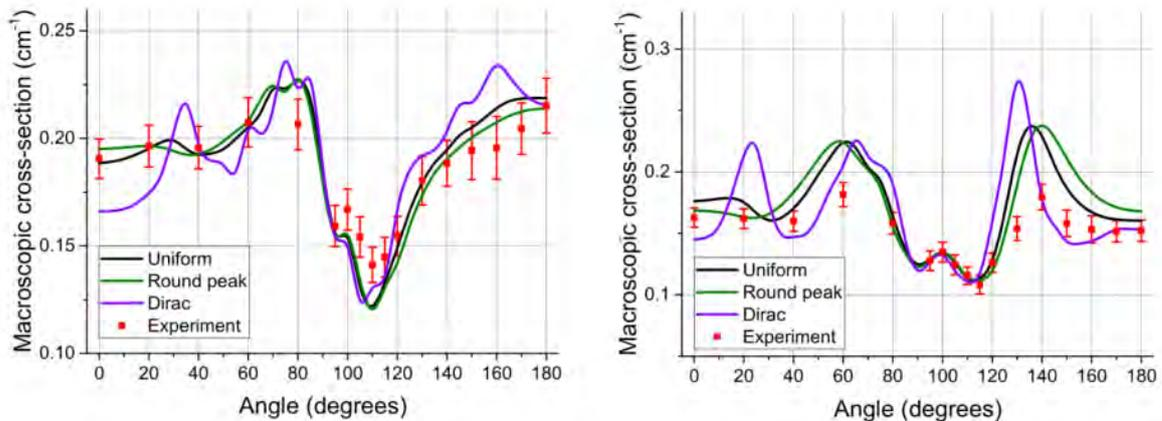
Figure 13. Experimental attenuation curves compared to simulated ones for three loading profiles for alumina (left) and magnesia (right).
