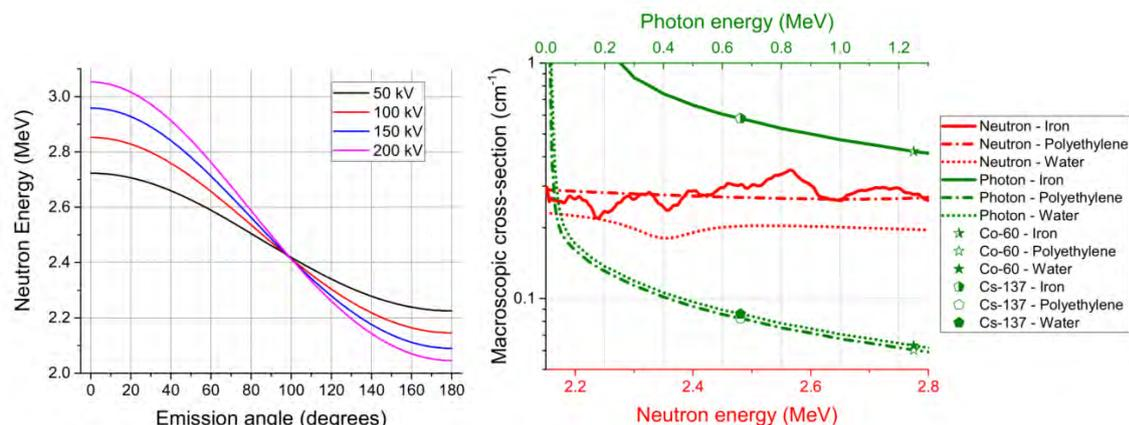
**Figure 1. Neutron energy vs. emission angle for different deuterium acceleration voltages (left) and the macroscopic attenuation coefficients for neutrons and photons for example materials in the energy regions of interest (right).**
