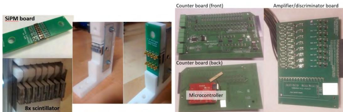
Figure 8. Photos of second-generation 8-detector module scintillator holder, SiPM-holder board, and readout electronics boards.
