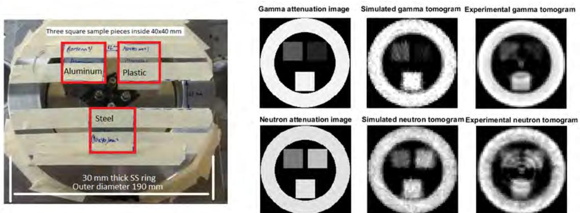
Figure 10. Sample object photo (left), theoretical attenuation image, simulated tomogram, and experimental tomogram for both Co-60 and fast neutrons (right).
