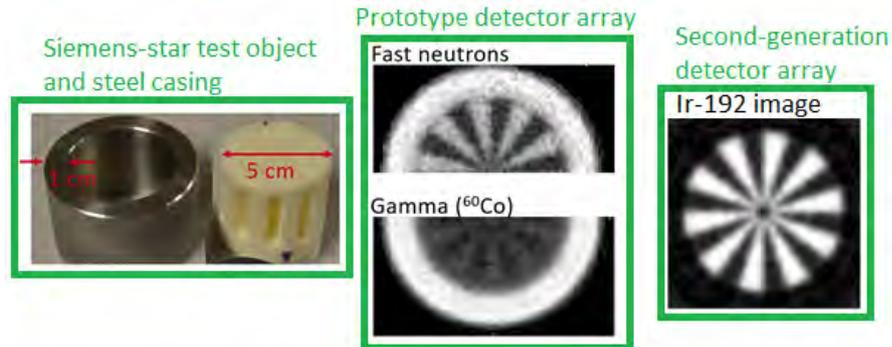
Figure 9. Photo and tomographic images produced by the prototype and second-generation detector array.
