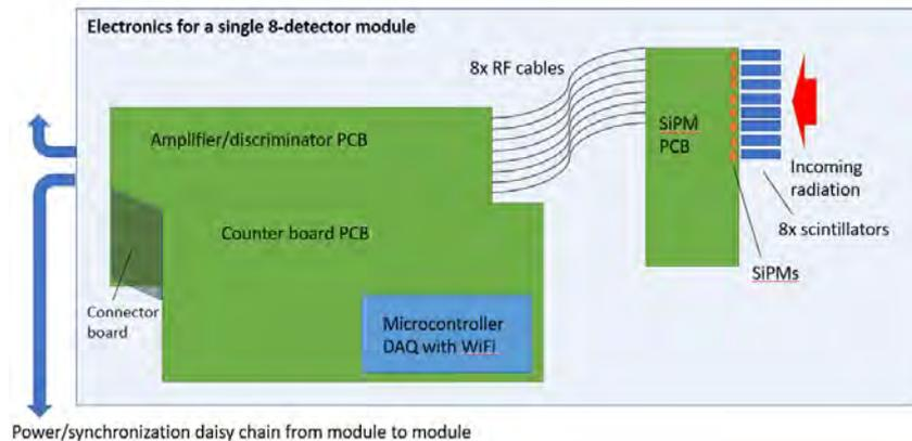
Figure 6. Schematic of 8-detector module.
