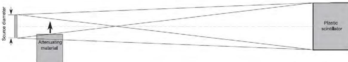
Figure 4. Schematic of edge spread measurement to determine emitting spot size.
