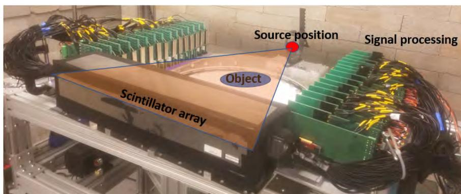
Figure 11. Completely assembled next-generation detector array to be applied to Ir-192 imaging.
