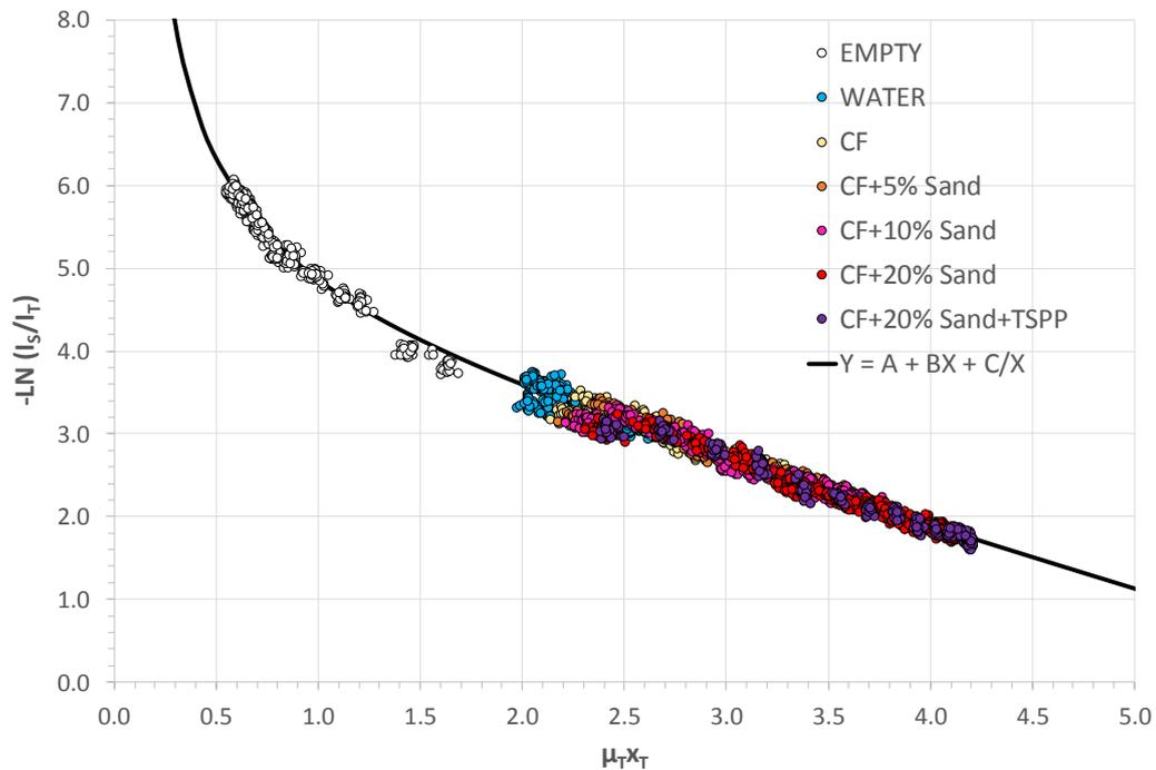
Figure 5. Normalized backscattering correction data for the high attenuation slurry measurements with the SRC GRT.
