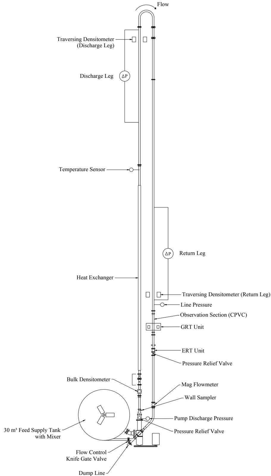
Figure 3. Schematic of the SRC 4 in. (100 mm) diameter recirculating pipe loop.
