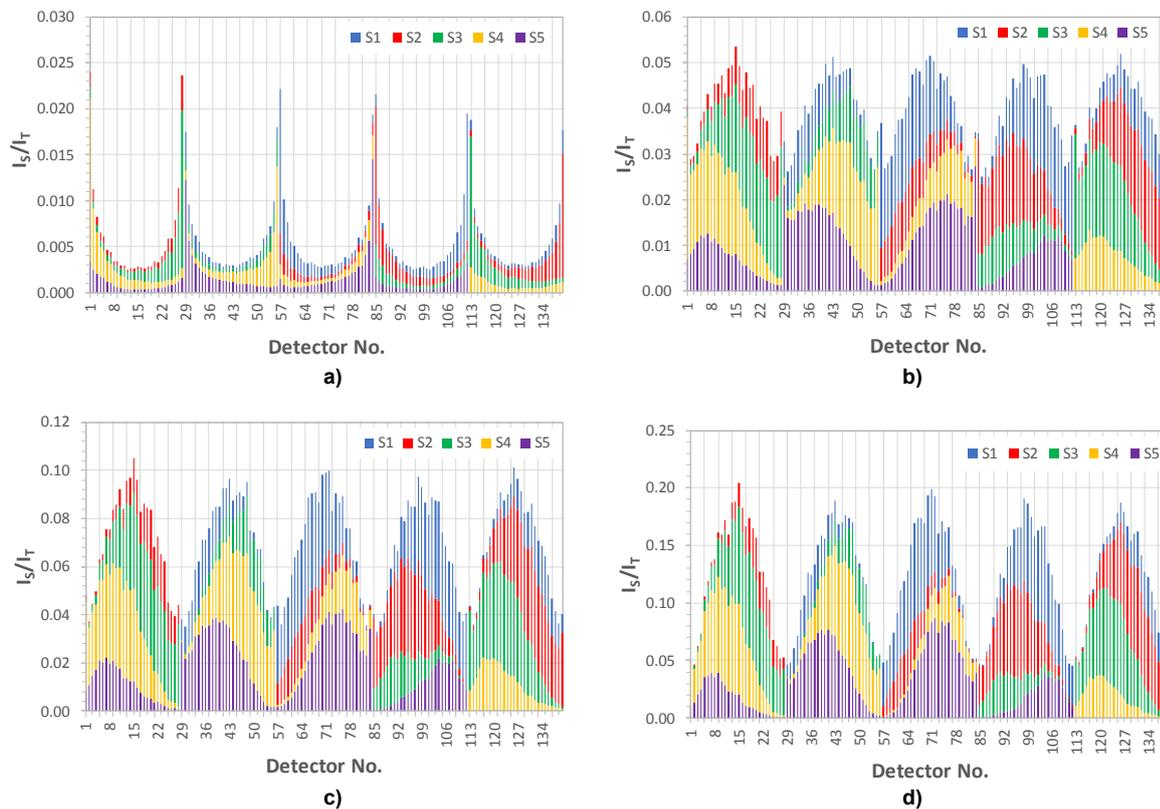
**Figure 4. Ratio of scattered to attenuated radiation intensity from the neighbouring sources at each detector: a) Empty Pipe, b) Water (998 kg/m<sup>3</sup>), c) Clay/Water Slurry (1282 kg/m<sup>3</sup>), d) Clay/Water/Sand Slurry (1580 kg/m<sup>3</sup>).**
